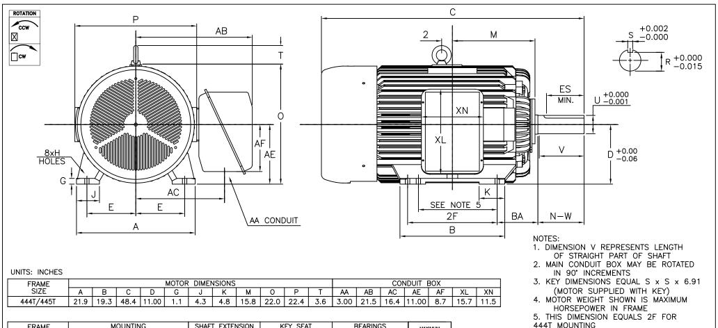
MOUNTING **BEARINGS** SHAFT EXTENSION KEY SEAT FRAME MAXIMUM SIZE ВА R S LS Н N-WU ES WEIGHT 444T/445T 9.00 | 14.50/16.50 | 0.81 7.50 | 8.50 | 8.25 | 3.375 | 2.875 | 0.875 | 6.91 | NU318C3 | 6318C3
